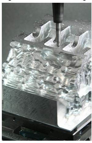
5 axis machining with the SINUMERIK MDynamics technology package
